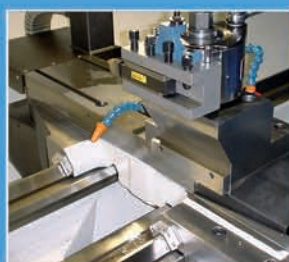
Large banc à 2 Vés de guidage | Large bed with 2 V-slides
